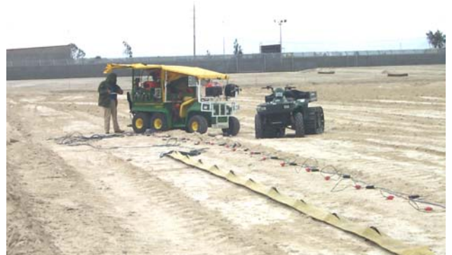
The KGS streamer is constructed from a fire hose. Shown here is the KGS recording system, consisting of a 240 channel StrataView mounted on an all-terrain vehicle.
