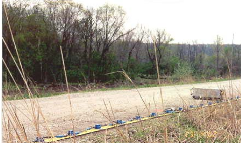
Bay's land streamer on a gravel road, imaging the subsurface using energy from Bay's shear-wave vibrator
