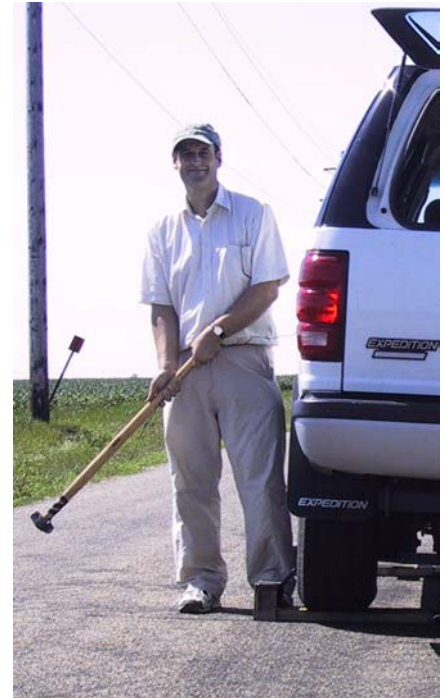
The IGS high frequency, high production rate seismic source, caught mid-swing.
