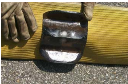
Geophones are mounted to a weighted cutter that creates a trench for better coupling
