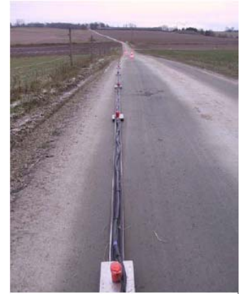
The long and winding road. Ramboll's land streamer moves fast and avoids permits
