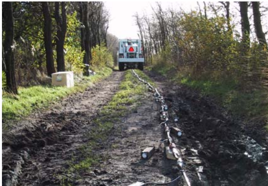
Gimbaled geophones on drop leads orient geophones and improve data quality on dirt roads
