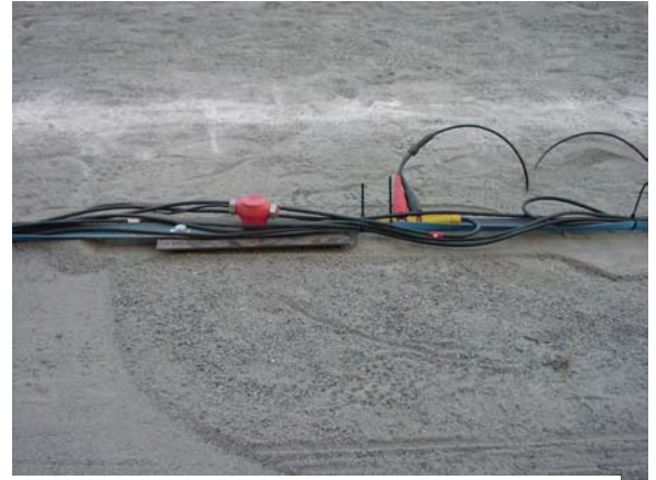
A simple metal plate provides good coupling for Tyrens surface wave surveys
