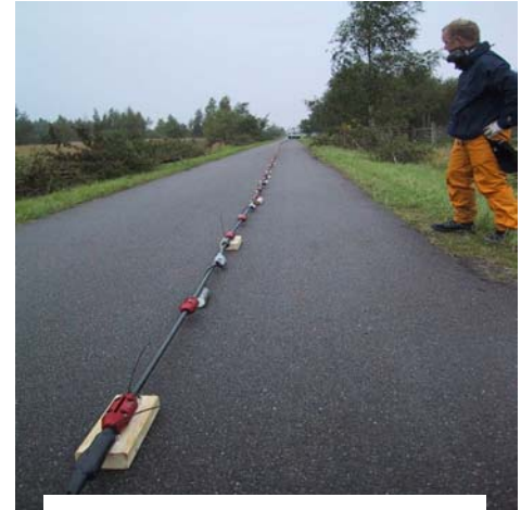
Wood blocks level streamer on pavement and reduce wear
