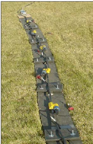
A weighted rubber mat, similar in construction to the ETH design, is used to eliminate cable tangles and improve coupling
