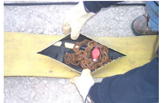
Weight can be added to the interior of the streamer to compensate for ground conditions
