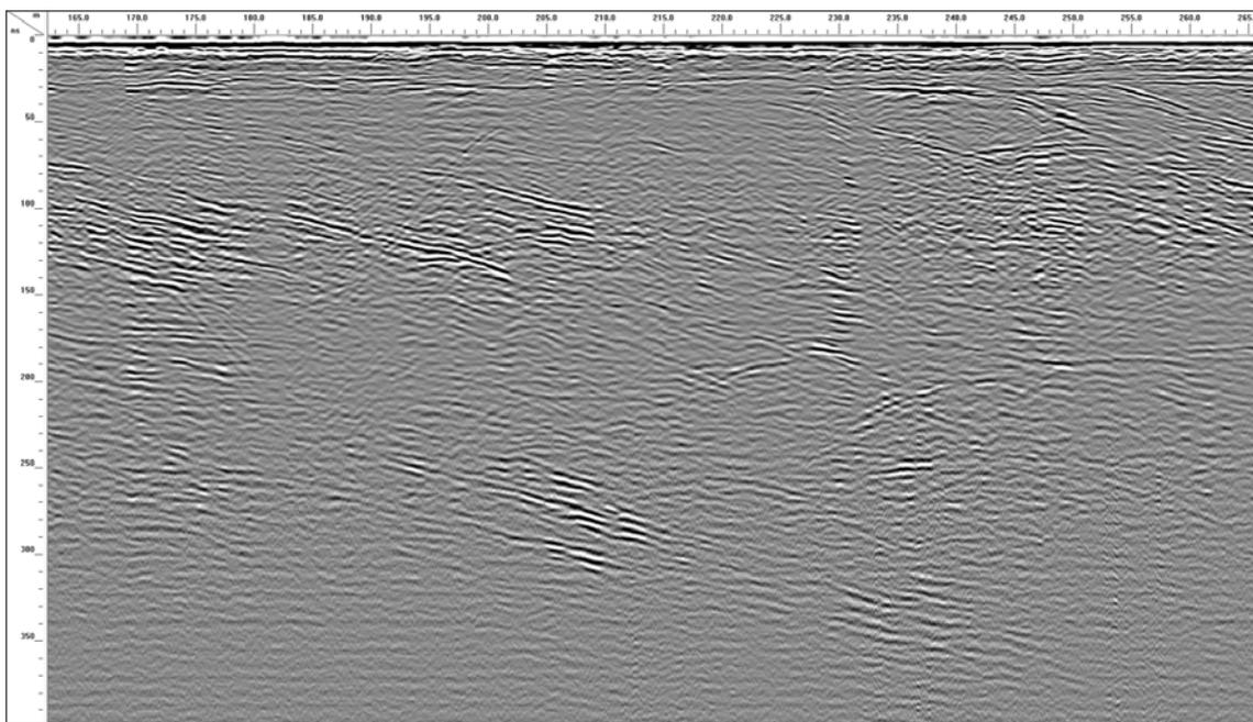
Data illustrates a terminal end moraine deposit with visible stratigraphy greater than 375 nanoseconds.
