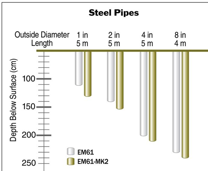
Figure 1: Depth of Detection for Steel Pipes
