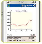
Stored data from RD8000 transferred by Bluetooth<sup>®</sup> may be displayed on a PC or PDA using Radiodetection's SurveyCERT<sup>™</sup> application
