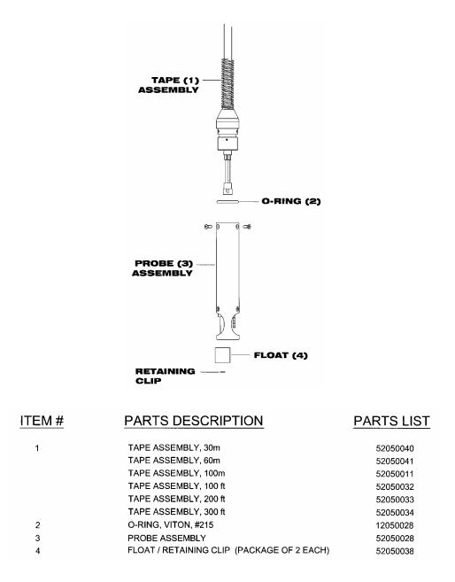
Figure 6 – Tape/Probe Parts List
