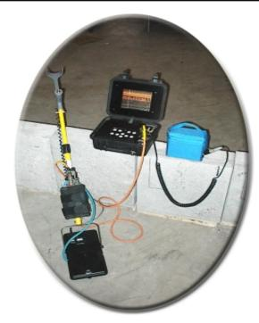
Specially configured for access to small areas. Used to locate objects embedded in concrete, such as rebars, tendons and conduit and other very high resolution, near-surface applications.
