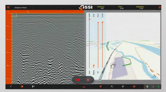
Tablet screen image of 2D GPR data indicitive of flood plain deposits located in the Northeastern United States (left) and geopgraphic information system (GIS) data (right).
