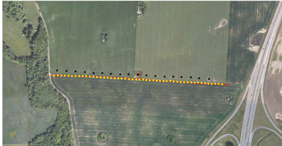
Figure 4 The map shows the National Danish Test site. Black dots: Aarhus University WalkTEM 40x40 m central coil measurement, 2010. Red line: ERT profile, 700 m long, 5 m electrode spacing, standard gradient protocol, 2023. Yellow dots: TEM2Go, 10 m sounding spacing, 2025. The central dot in the middle is the test site, while the dots along the line are the test line. Reference: Test-site calibration and validation of airborne and ground-based TEM systems. N Foged, E Auken, AV Christensen, KI Sørensen - Geophysics, 2013
