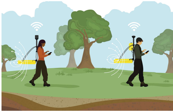
Figure 1. The sketch shows the TEM2Go system. The transmitter is in front while the receiver is at the back. The distance between the coils is a minimum of 15 m.
