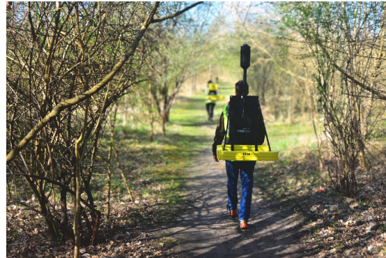
Figure 2. The TEM2Go system in operation.
