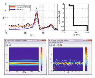
VIBRATION ANALYSIS. Sorting and spectral analysis of signal sections above thresholds, according to the European regulations on strong vibrations in structures. Automatic editable reports including tables and figures.
