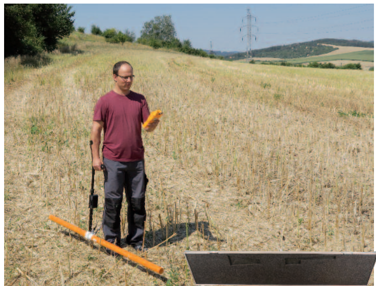
CMD - 4 single-depth probe with 6.0 / 3.0 m depth range with wide sphere of applications (geological survey, mapping of pollution plumes, raw material prospecting).
