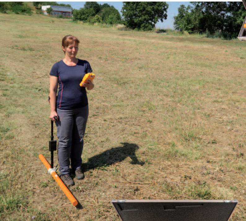
CMD-Explorer three-depth probe with depth ranges 2.2 / 1.1 m, 4.2 / 2.1 m, 6.7 / 3.3 m for extra wide range of applications with evaluation of vertical and horizontal conductivity changes.
