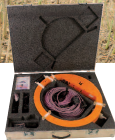
CMD - DUO single-depth, two-men operated probe with variable depth range 15 / 7.5 m or 30 / 15 m or 60 / 30 m for measurement of deeper situated structures (weathered zones, bedrock, cavities).
