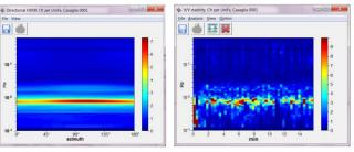
VIBRATION ANALYSIS. Sorting and spectral analysis of signal sections above thresholds, according to the European regulations on strong vibrations in structures. Automatic editable reports including tables and figures.
